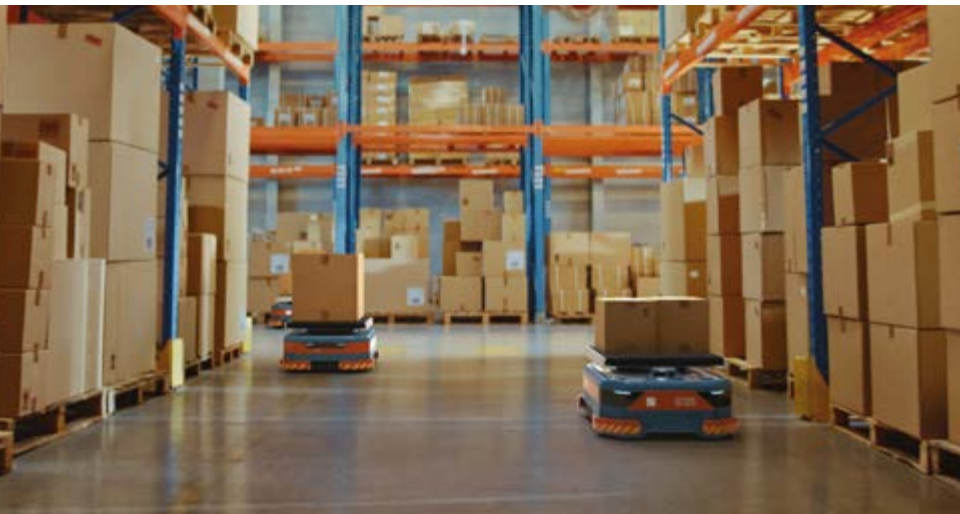
Food processors have begun to implement automated guided vehicles to move product around plants and warehouses. Use of similar technologies will help the food plant of the future be safer and more efficient.
